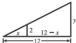
We are given that  $\frac{dx}{dt} = 1.6$  m/s. By similar triangles,  $\frac{y}{12} = \frac{2}{x} \Rightarrow y = \frac{24}{x} \Rightarrow \frac{dy}{dt} = -\frac{24}{x^2} \frac{dx}{dt} = -\frac{24}{x^2}(1.6)$ . When  $x = 8$ ,  $\frac{dy}{dt} = -\frac{24(1.6)}{64} = -0.6$  m/s, so the shadow is decreasing at a rate of 0.6 m/s.
